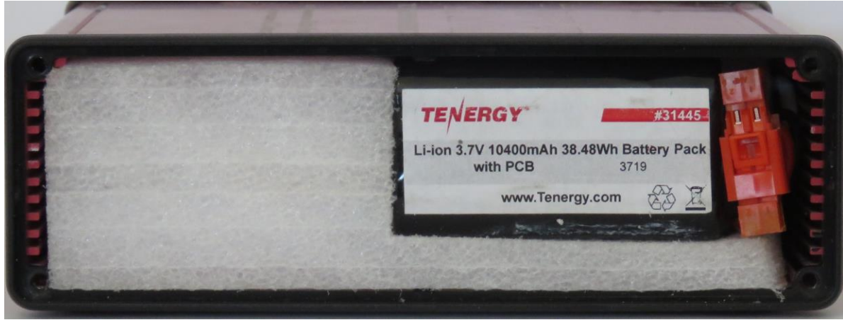
TKMD Backup Battery (Battery Access Cover Removed)
