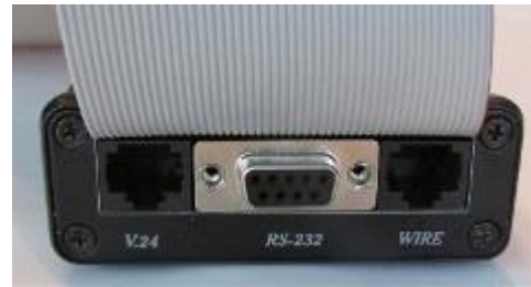
Stand-Alone RIC-Mz with Optional Ribbon Cable for connection to an ATAC-3000™, PDR-3500™ or Quantar™ without a V.24 Board
