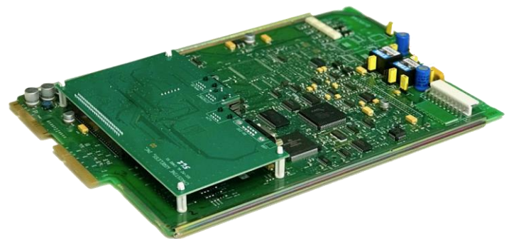
RIC-Mz Wireline Card installed on a Quantar™ Wireline Board that lacks a V.24 board
