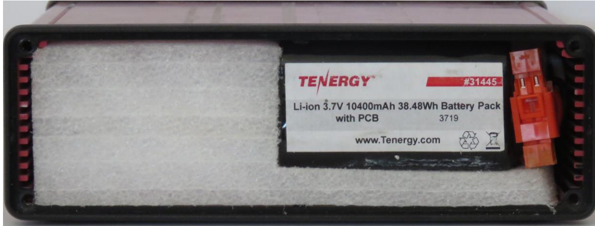
TKMD Backup Battery (Battery Access Cover Removed)
