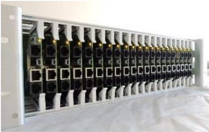
Card Cage for up to 21 RIC-Ms with redundant power supplies
