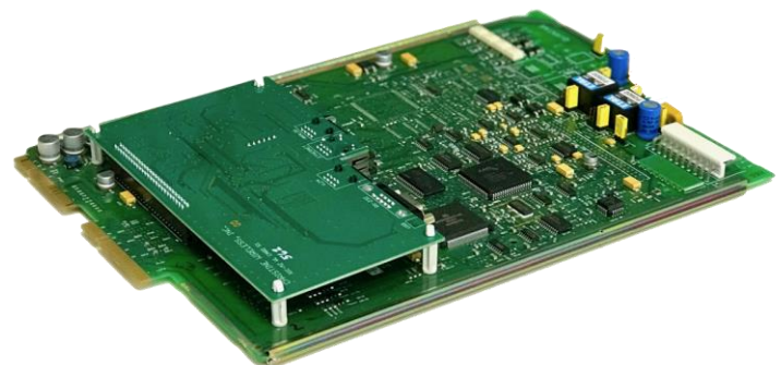
RIC-M Wireline Card installed on a Quantar™ Wireline Board that lacks a V.24 board
