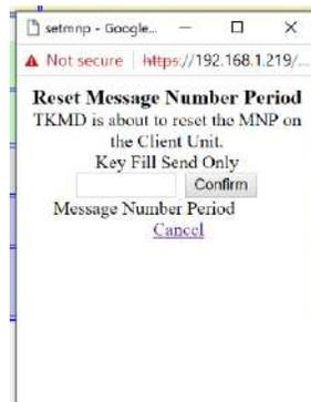
The desired MNP (up to 65535) is entered in the window and confirm is clicked to send the KFD command.
