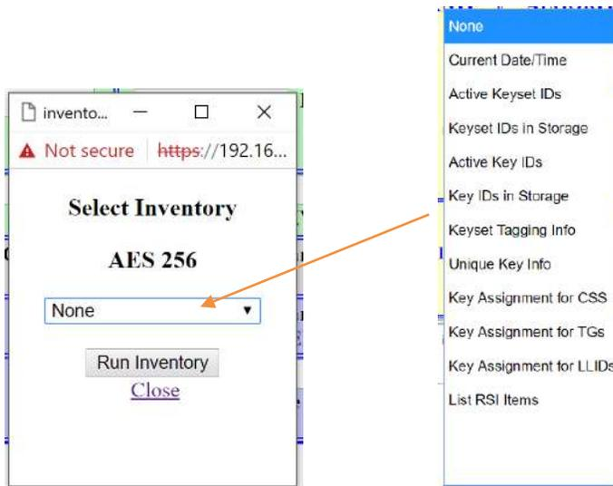
The Inventory type pulldown menu lists the possible types of inventories for the TKMD Operating mode. Not all types of inventory actions will be successful due to the wide range of differences between manufacturers in implementing OTAR standard features.
