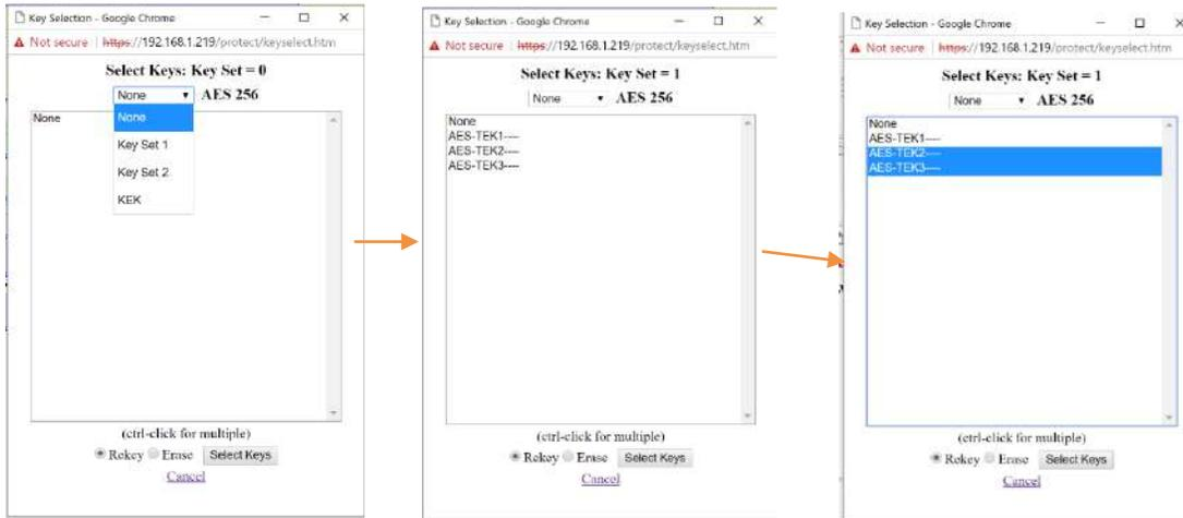
The Keys to be included in the Rekey Erase process, whether the action is Rekey or Erase and clicking the Select Keys button caused the indicated action to take place. Multiple keys can be selected by using shift or ctrl click. This window is used to select keys for both the OTAR and KFD operational modes.
