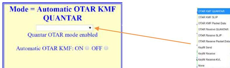
If Automatic OTAR KMF is desired, click the button for ON and then select one of the three options for OTAR KMF. If the TKMD is to be left in Automatic OTAR KMF (the normal
