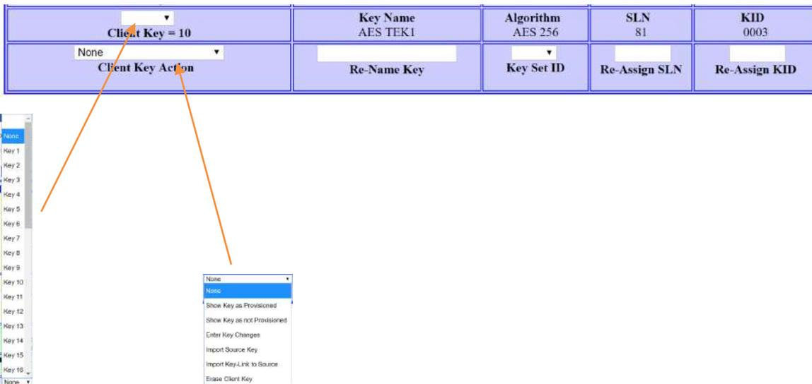
The Client Key Action pulldown menu is used to execute the desired action on the Selected Source key for the Selected Client target key location. If changes are desired for the Key Name, Key Set ID, SLN or KID, the changes can be entered in the appropriate entry block and they will be saved to the Client Selected target key location.
