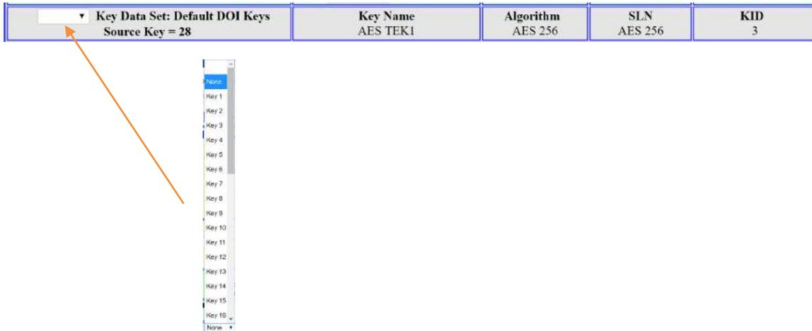
The Key Name, Algorithm Storage Location Number (SLN) and Key Identification (KID) parameters will be displayed for the selected key.
